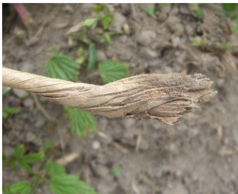
Fig. 5.5: Paper string that has rotted in the soil-air transition zone
