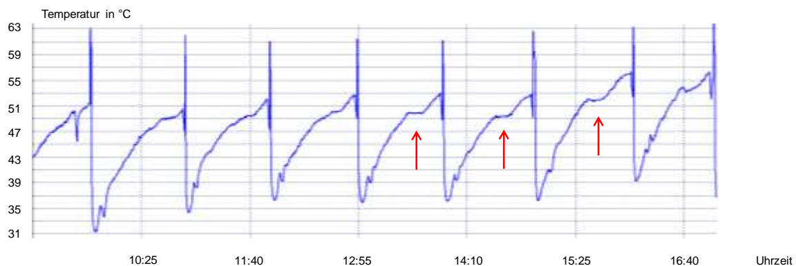
Fig. 5.22: Changing temperatures at the surface of the hop cones on the intermediate drying tier
