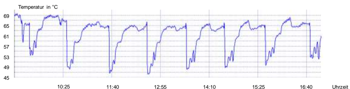
Fig. 5.23: Changing temperatures at the surface of the hop cones on the movable tier
