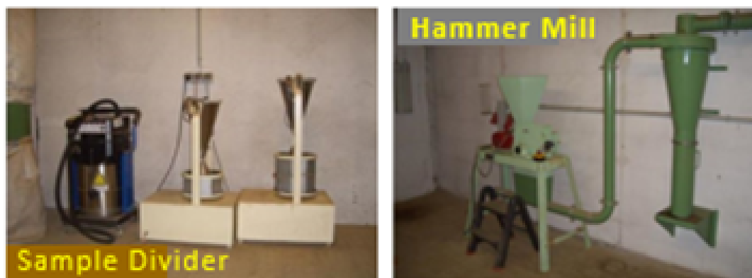
Figure 7.15: Sample divider and hammer mill
