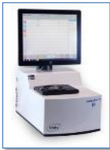
Figure 7.20: NIRS device from Unity Scientific
