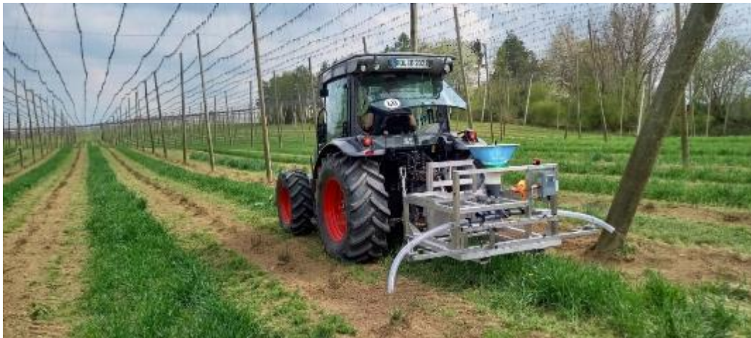
Figure 8.4: Modified construction of a device by Koppert for the early application of predatory mites close to the ground in hop gardens in Dürnwind on May 2, 2022
