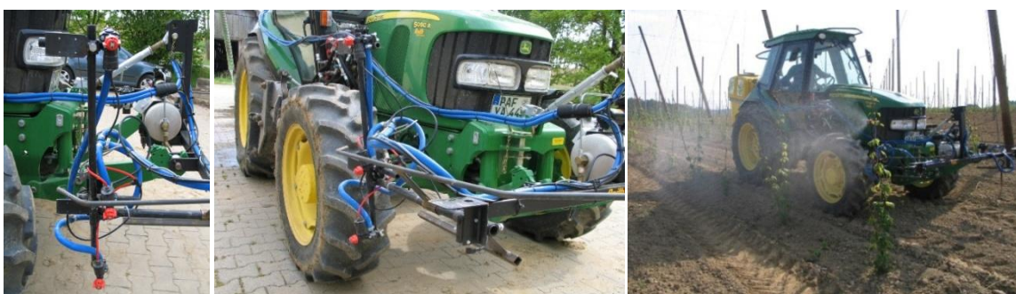
Fig 5 - 7: Sensor-controlled application technique for the second time of application (02/05/2011) to 1.5 m height
