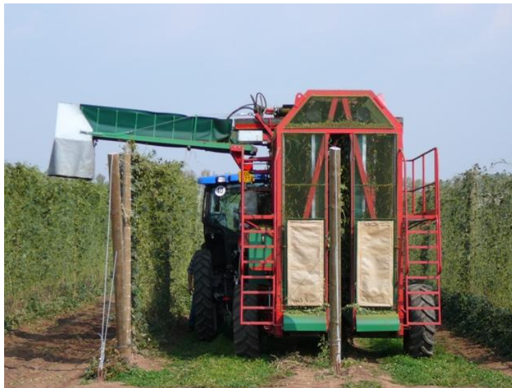
Fig. 1: Permanent grassing in low trellis helps the smooth operation of mobile harvester HUN-30 (photo by J. Ježek)
