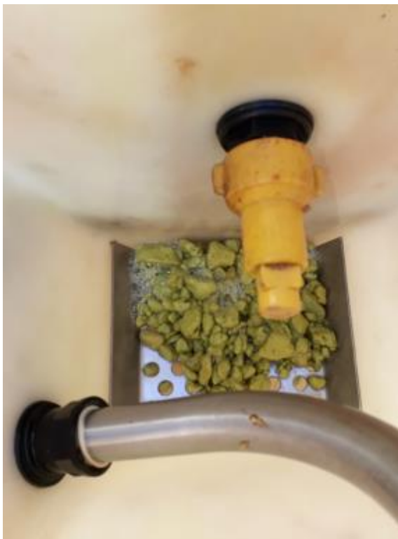
Fig. 8.6: Direct filling of the sprayer with hop caps without first stirring them in water continued to form lumps
