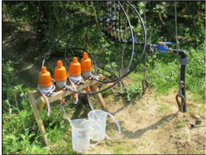
Fig. 4.3: Fertilizer dispensing device for fertigation
