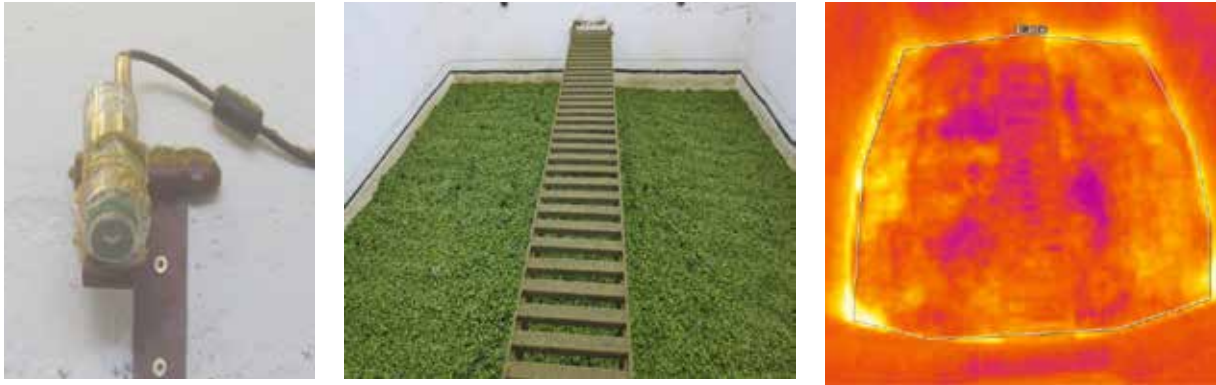
Fig. 4.11: Thermal imaging camera; measuring surface on top of the hop bed in the kiln; thermal measurement image
