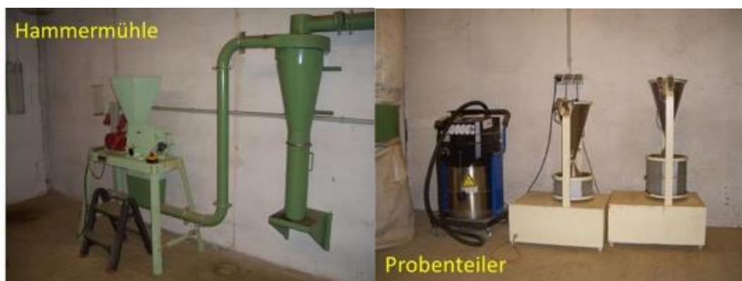
Figure 7.20: Hammer mill ( Hammermühle ) and sample divider ( Probenteiler )
