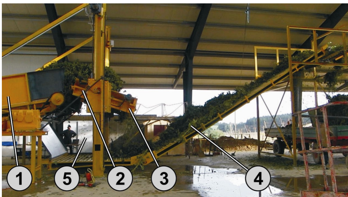
Figure 3 Prototype of the system for automated feeding of the picking machine. Legend: (1) – conveyor; (2) – mechanism for cutting; (3) – pre-picking unit; (4)– feeding mechanism; (5) – electrical cabinet with the PLC
