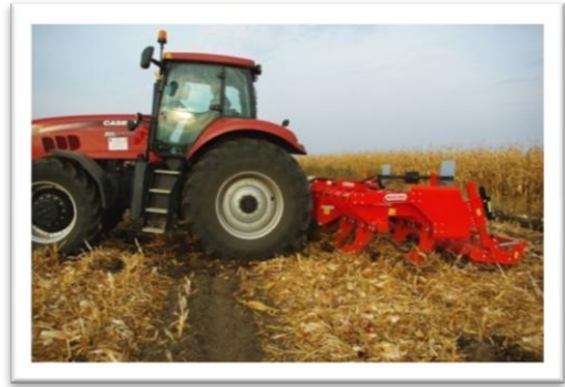
Grubber with crumbler roller, 0.25 m working depth
