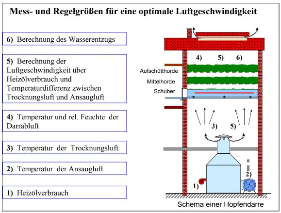
Fig. 5.2: Required drying parameters for the fully automated air-speed meter
