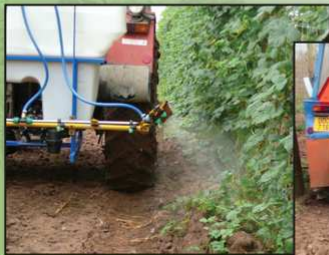
Example: machine for chemical regulation of hop growth and for mechanical cutting
