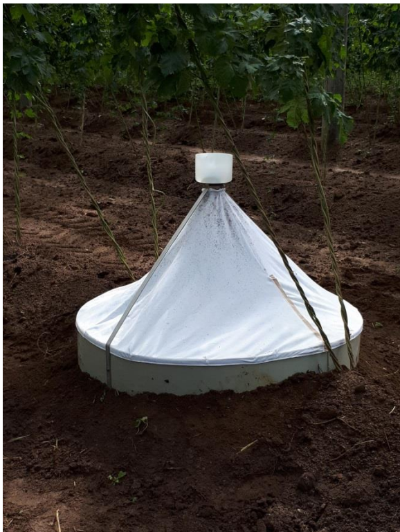
Fig. 7.4: Installation of the photo eclectors in the middle of each plot in the trial yard.
