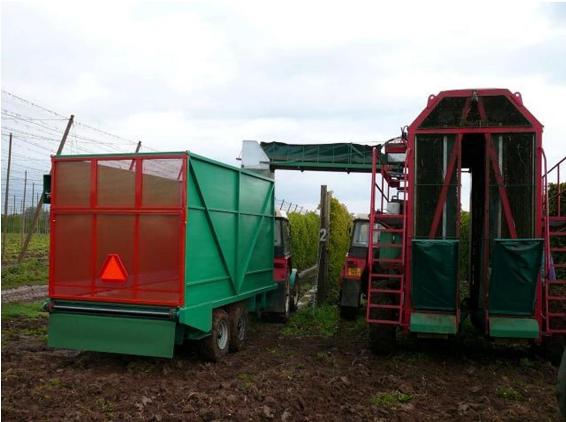
**Figure 1.** Special trailer for hop mass and mobile hop picking machine HUN-30
