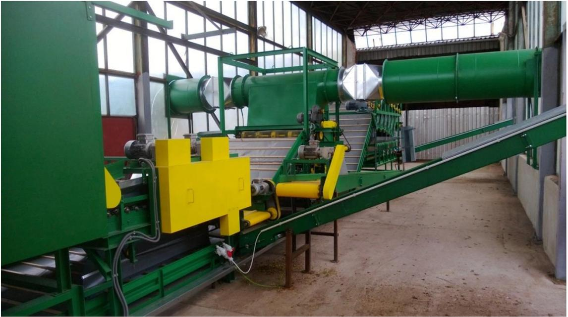
**Figure 4.** The new design of a PT-2000 cleaning line for low trellis
