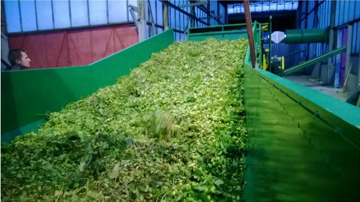
**Figure 3.** Loading conveyor ('feeding table') of a new PT-2000 cleaning line for low trellis
