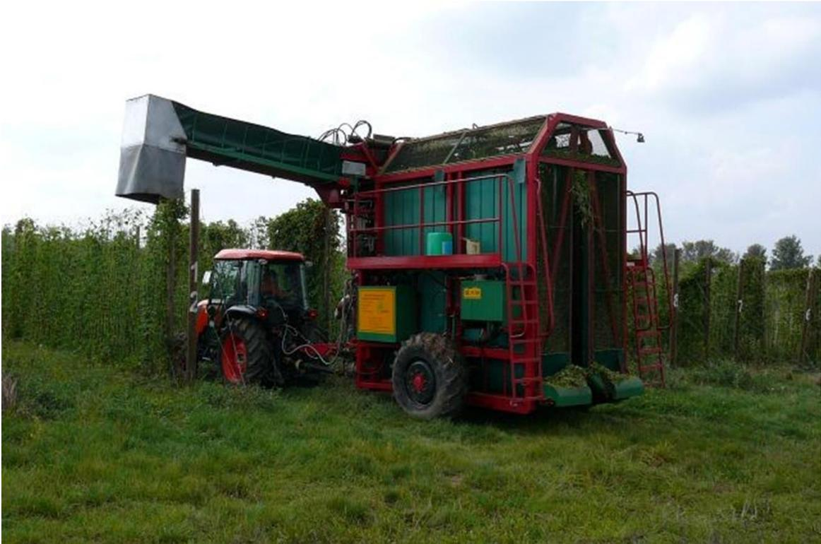
**Figure 2.** Mobile hop picking machine HUN-30 in a low trellis system in the Saaz hop growing region
