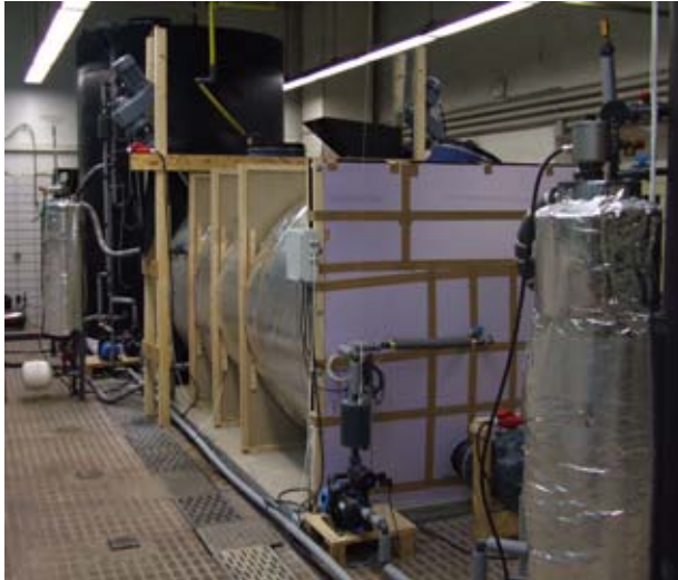
Fig. 6: Test plant ISAH 1 m 3 hydrolysis, 105 L UASB reactor
