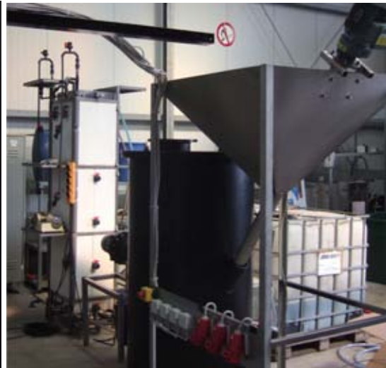
Fig. 7: Test plant TiHo 5 m 3 hydrolysis, 10 m 3 methane reactor
