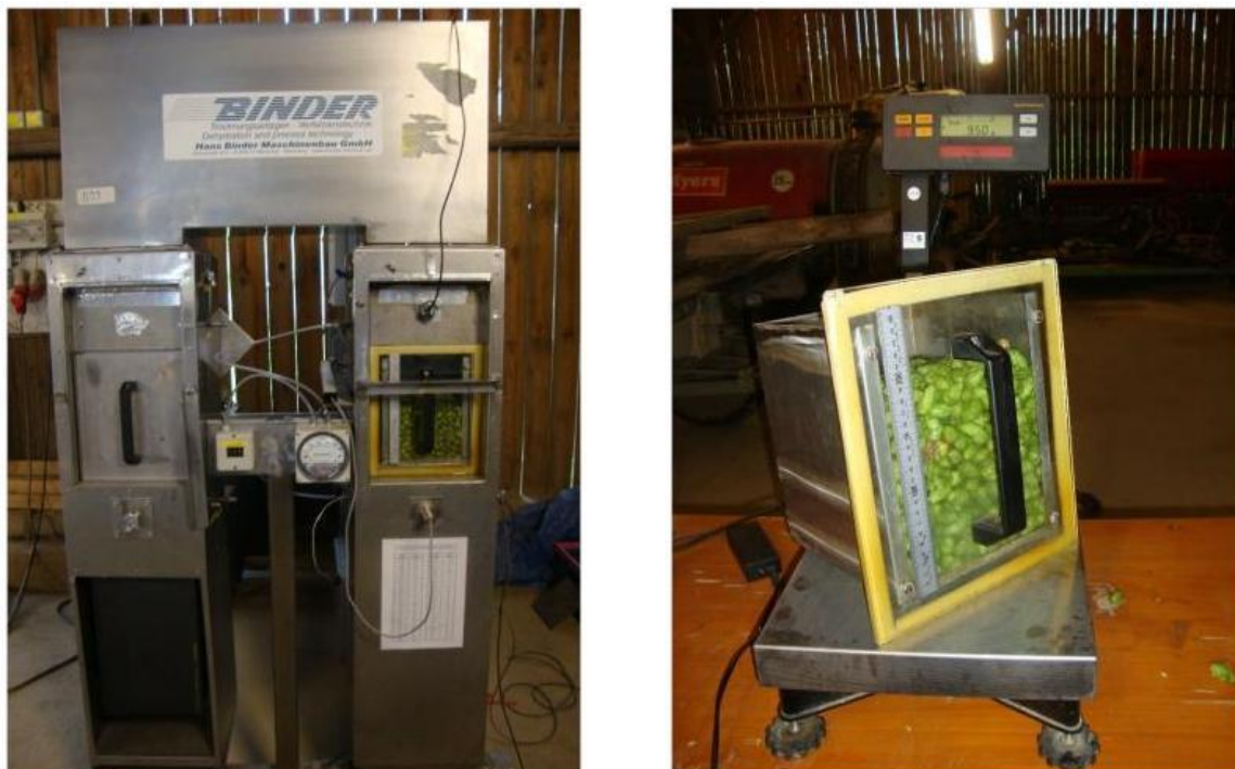
Fig. 5.3: Small-scale drying-trial setup (left) and weighing device (right) for measuring water extraction during drying
