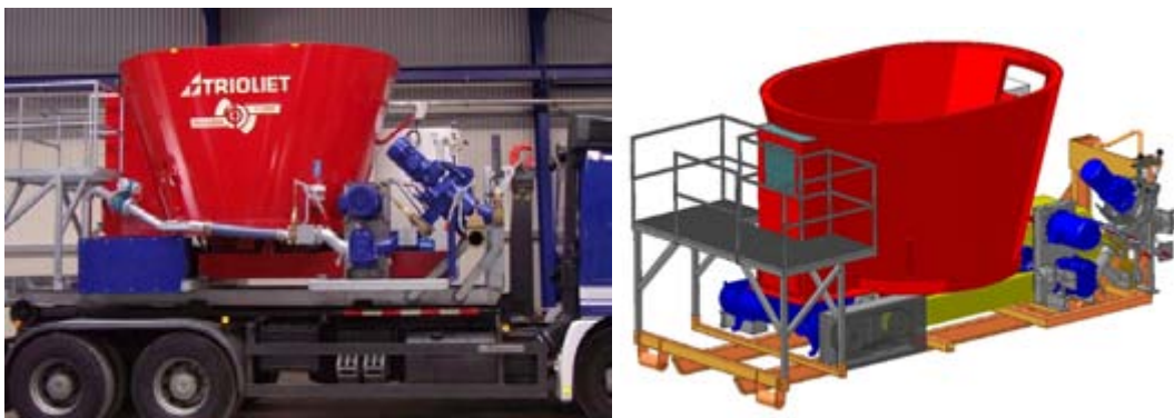
Fig. 2: Mobile mixing/feeding unit
