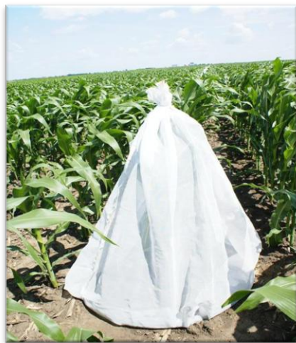
Hatch cages, 1.4 m height, covering a ground surface of 1 m 2 , with gauze clothing
