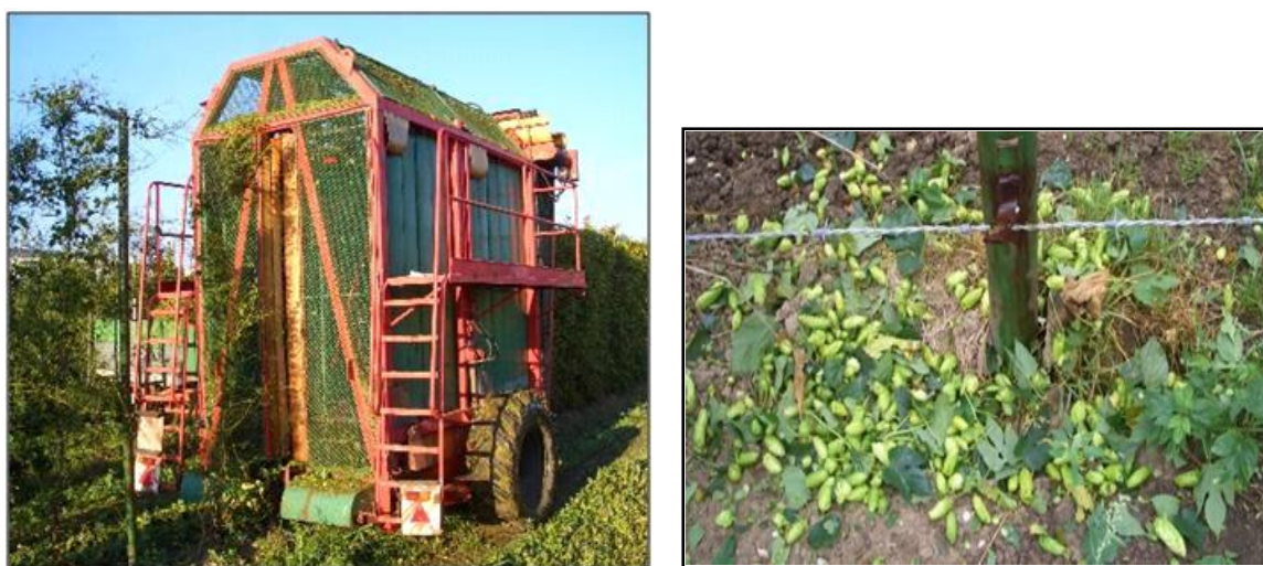
Fig. 4.1. : The mobile picking machine harvesting hops (left). Losses of harvested hop cones around the posts (right) were substantially reduced in 2010 thanks to a number of improvements to the mobile picker.
