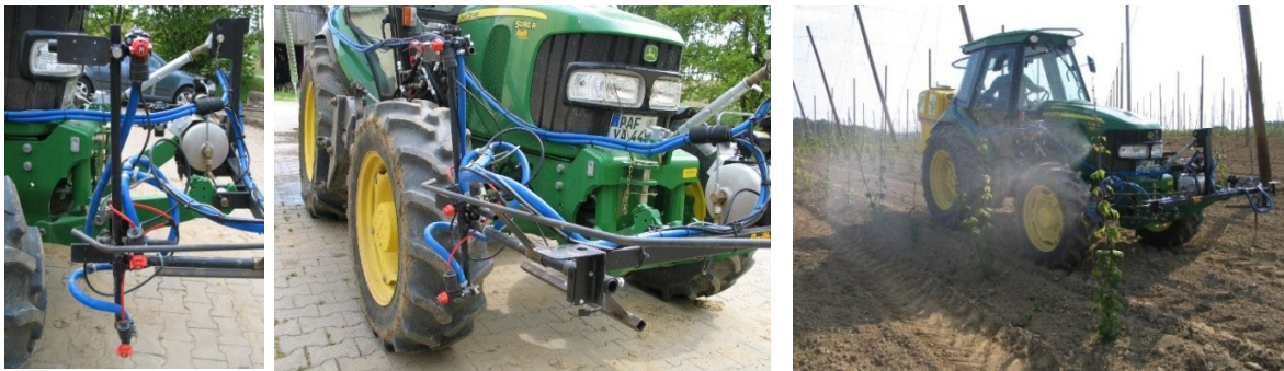
Fig. 5.25, Fig. 5.26 and Fig. 5.27: Sensor-controlled application technique for follow-up spraying (02.05.2011) up to 1.5 m in height
