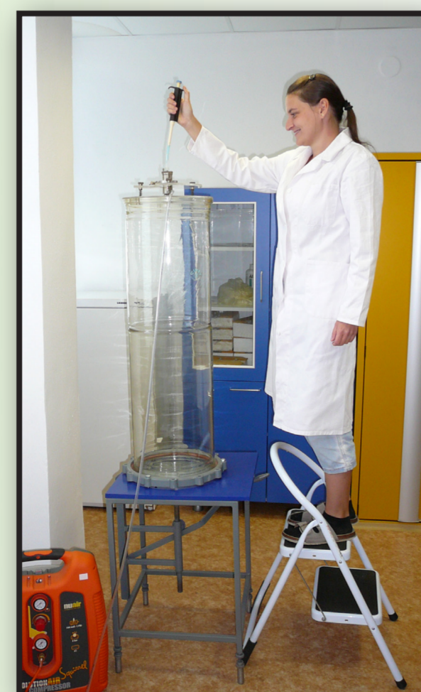
FIGURE 5: Hop leaves placed at the bottom of the sedimentation tower are treated with Teppeki applied in a geometric row of tested concentrations
