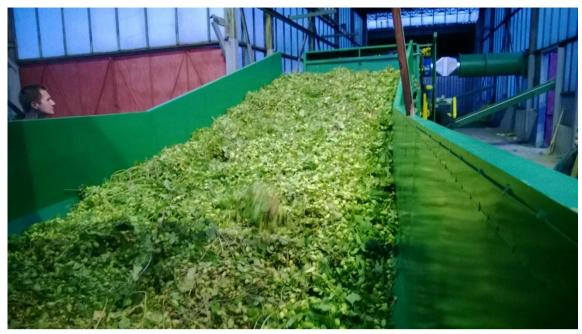
Figure 3. Loading conveyor ('feeding table') of a new PT-2000 cleaning line for low trellis
