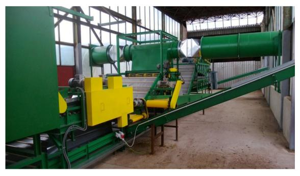
Figure 4. The new design of a PT-2000 cleaning line for low trellis
