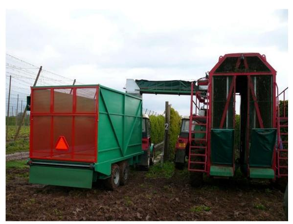
Figure 1. Special trailer for hop mass and mobile hop picking machine HUN-30
