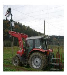
while watering with pesticides. By utilizing optical sensors in combination with special nozzles the amount of pesticides could be reduced drastically, since the nozzles only opened when the bine or wire were recognized
